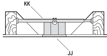
To hang your fan where there is an existing fixture but no ceiling joist, you may need an installation hanger bar (KK) (not included) as shown above.
